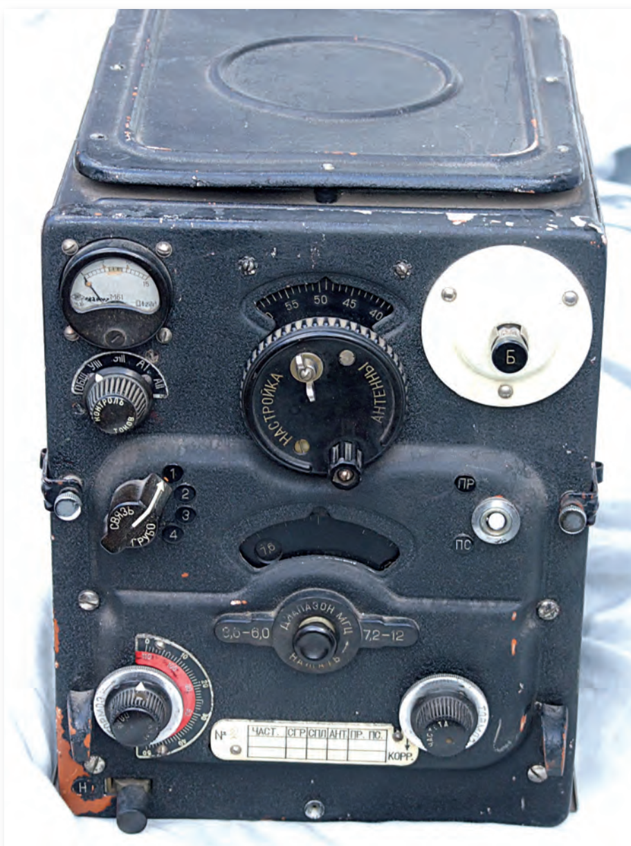
Fig. 3: The Russian transmitter RSB-5, the band switch is a push-pull switch mounted at the lower centre of the unit.
