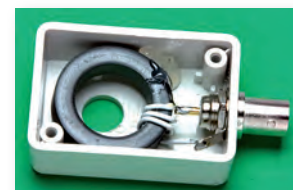
Fig. 3: The unusual method of coupling into the loop winding.
