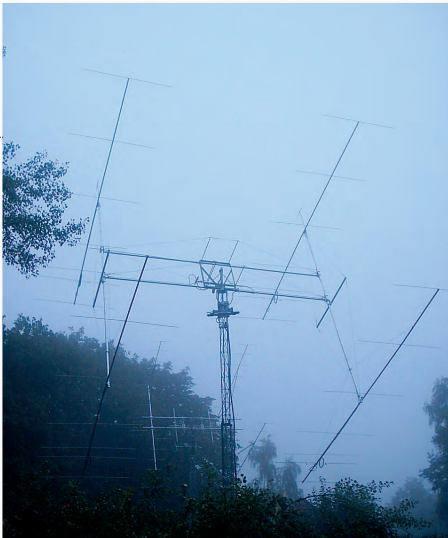
Fig. 1: The 50MHz EME Station at PE1BTX. It consists of four 6M7JHV, 7-element Yagi antennas.
