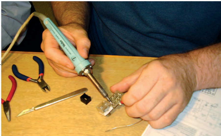
An older temperature controlled soldering iron, such as this Weller 24V iron can often be found at rallies. But do try to check that it works first.
