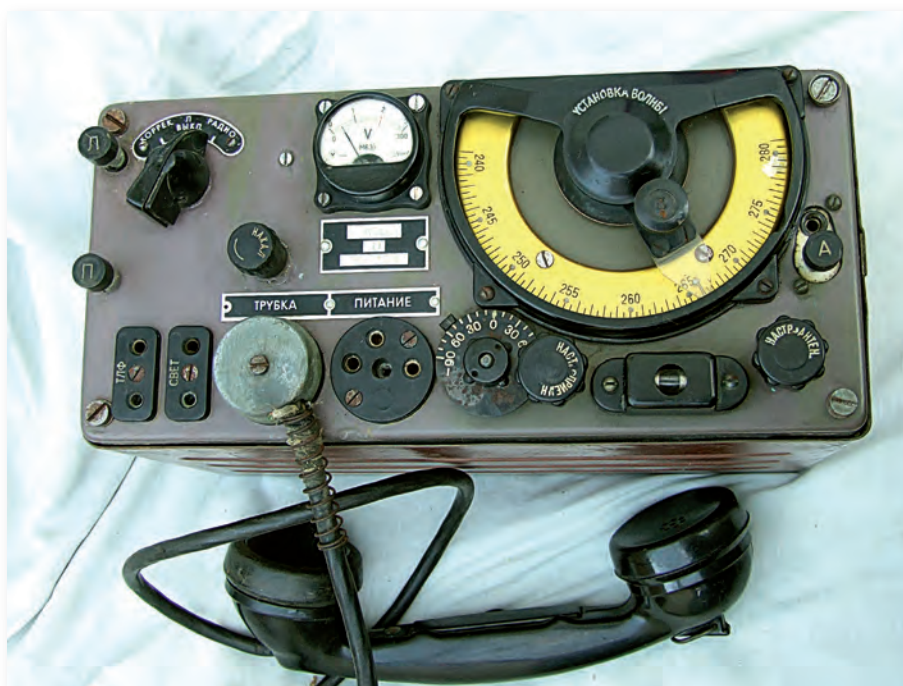
Fig. 4: The A7b transceiver. This version came with a telephone type microphone-headset.
